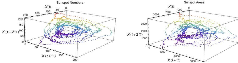
**Fig. 5** Plots of reconstructed phase spaces with the estimated parameters for smoothed monthly-mean SNs (*left panel*) and SAs (*right panel*).
